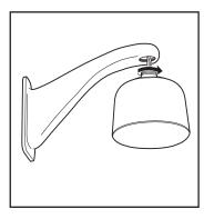
d. Screw the back box into the mount. If outdoors, apply thread compound (provided) to the threads on the back box.
